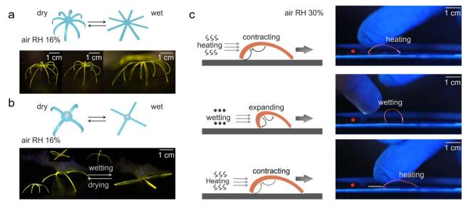
Fig. 6 Applications of hybrid organic crystals. (a) Illustrative diagram and photographs showing a soft robot designed to mimic spider-like movements. (b) Diagram and images of a soft gripper constructed from hybrid organic crystal. (c) Schematic and photographs depicting the 'walking' movement of organic polymer-crystal hybrid materials on a surface. (a–c) Reproduced with permission from ref. 27, Copyright 2023 Spring Nature.
