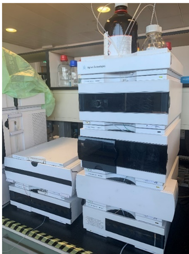
Fig. 4 Typical HPLC set-up that can be adapted for use in continuous flow processes.
