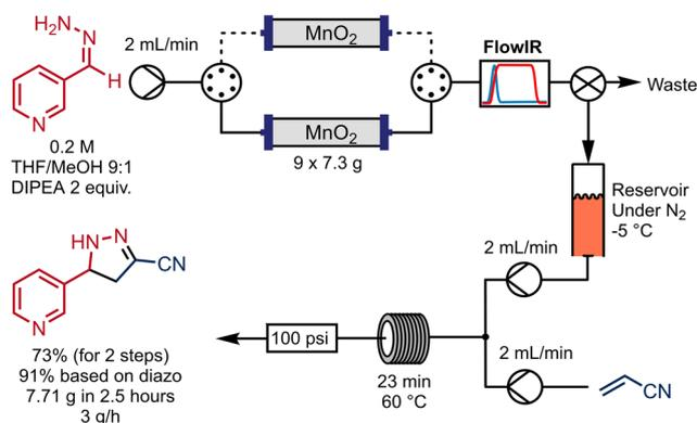
**Scheme 5** Multi-column setup for scale out of the pyrazoline synthesis using a pre-conditioned MnO<sub>2</sub> columns.
