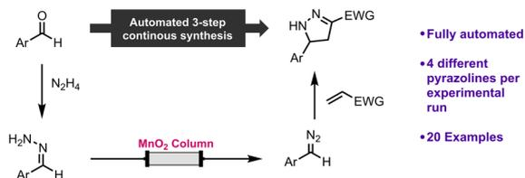
**Scheme 1** Previous work handling unstabilised diazo compounds (a) and this work on the multi-step synthesis of 2-pyrazolines from aldehydes (b).
