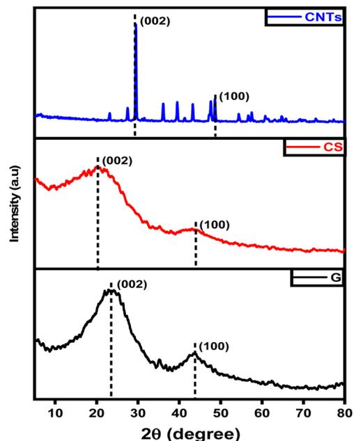
Fig. 3 XRD patterns of graphene, carbon spheres, and carbon nanotubes.
