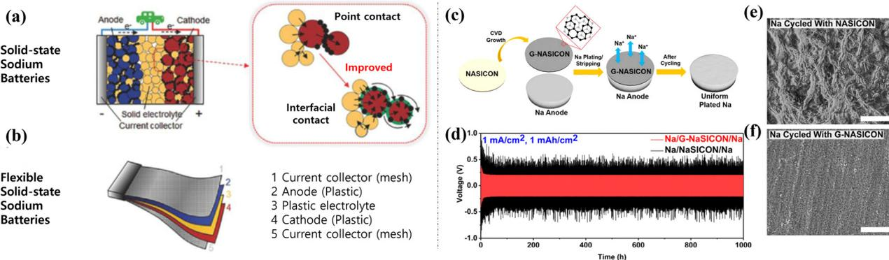
**Fig. 14** Illustration of (a) solid-state sodium batteries and (b) flexible solid-state sodium batteries. Reprinted with permission from ref. 164. Copyright 2021 American Chemical Society. (c) ASSSIBs prepared with ultrathin graphene layer-NASICON. (d) Na stripping/plating cycling performances with (e) graphene layer-NASICON and (f) conventional NASICON and their surface morphologies. Reprinted with permission from ref. 165. Copyright 2019 American Chemical Society.
