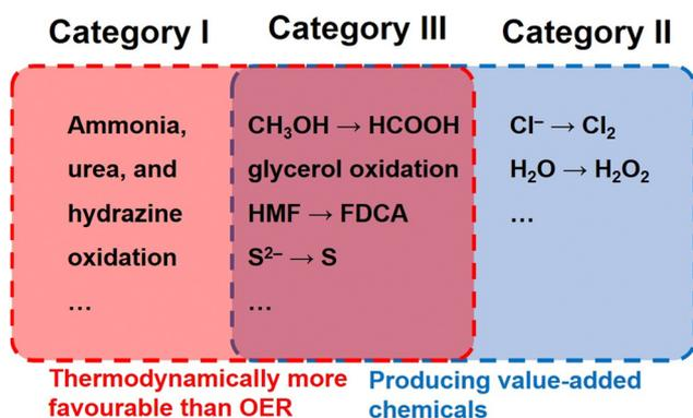
**Fig. 1** Different categories of alternative anodic oxidation reactions.
