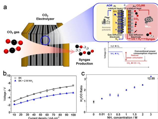
Fig. 2 (a) Schematic illustration of the  $\text{CO}_2\text{RR}$ -AOR couple in a gas diffusion electrolyser. (b) Voltages at different current densities in 0.5 M  $\text{KHCO}_3$  (BK) or 0.5 M  $\text{KHCO}_3 + 2 \text{ M NH}_3$  (BK + 2 M  $\text{NH}_3$ ). (c)  $\text{H}_2/\text{CO}$  ratio of syngas as a function of the  $\text{NH}_3$  concentration at  $10 \text{ mA cm}^{-2}$ . Reproduced with permission from ref. 30. Copyright 2022, Elsevier Ltd.
