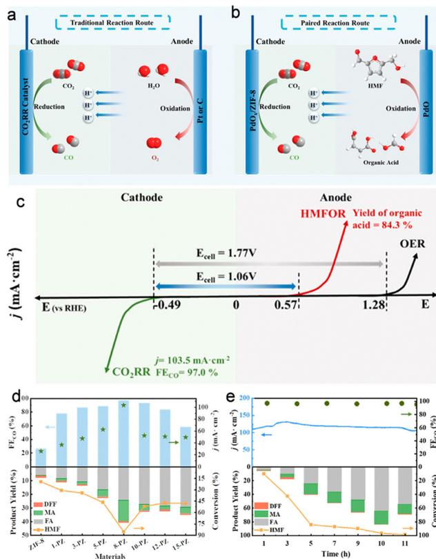
Fig. 7 Overview of (a) CO<sub>2</sub>RR-OER and (b) CO<sub>2</sub>RR-HMFOR routes. (c) Comparison between the CO<sub>2</sub>RR-OER and the CO<sub>2</sub>RR-HMFOR. (d) CO<sub>2</sub>RR and HMFOR performances with different anodic catalysts. (e) Long-term electrolysis results of the CO<sub>2</sub>RR and HMFOR. Reproduced with permission from ref. 19. Copyright 2022, American Chemical Society.
