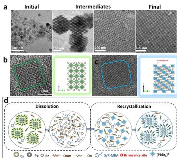
**Fig. 4** Transient phases in the conversion of CsPbBr<sub>3</sub> to Cs<sub>4</sub>PbBr<sub>6</sub>: (a) TEM images of the initial Br perovskite NCs and of intermediates upon conversion to the final Cs<sub>4</sub>PbBr<sub>6</sub> product. TEM images and atomic model (b) of cubic CsPbBr<sub>3</sub> (c) and of rhombohedral Cs<sub>4</sub>PbBr<sub>6</sub> NCs. (d) Schematic of the proposed dissolution–recrystallization transformation mechanism.
