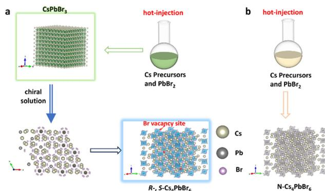
**Fig. 1** (a) Schematic of the phase transformation from 3D cubic CsPbBr<sub>3</sub> to hexagonal OD *R*- and *S*-Cs<sub>4</sub>PbBr<sub>6</sub> NCs. (b) Schematic of the synthesis of N-Cs<sub>4</sub>PbBr<sub>6</sub> NCs.
