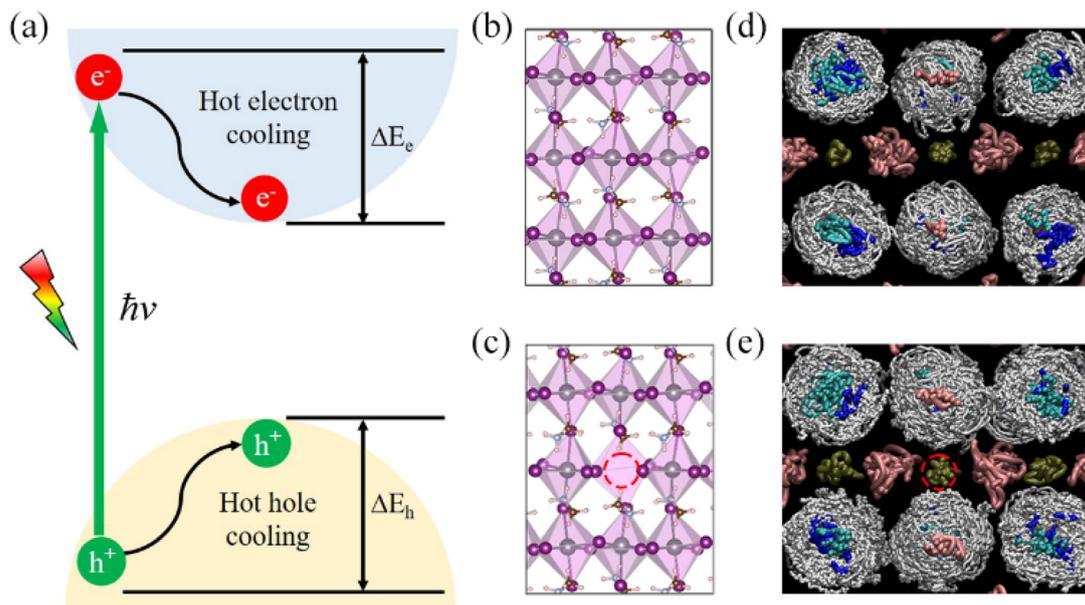
**Fig. 1** Schematic illustration of hot carrier relaxation (a). Optimized ground state structures of pristine MAPbI<sub>3</sub> (b) and MAPbI<sub>3</sub> with Pb<sub>v</sub> (c). Superimposed snapshots of local structures from 5 ps molecular dynamics trajectories of pristine (d) and defective (e) MAPbI<sub>3</sub>. The red dashed circle denotes the location of vacancy site. The motion of MA cations in the defective system is enhanced due to the additional space created by Pb vacancies.
