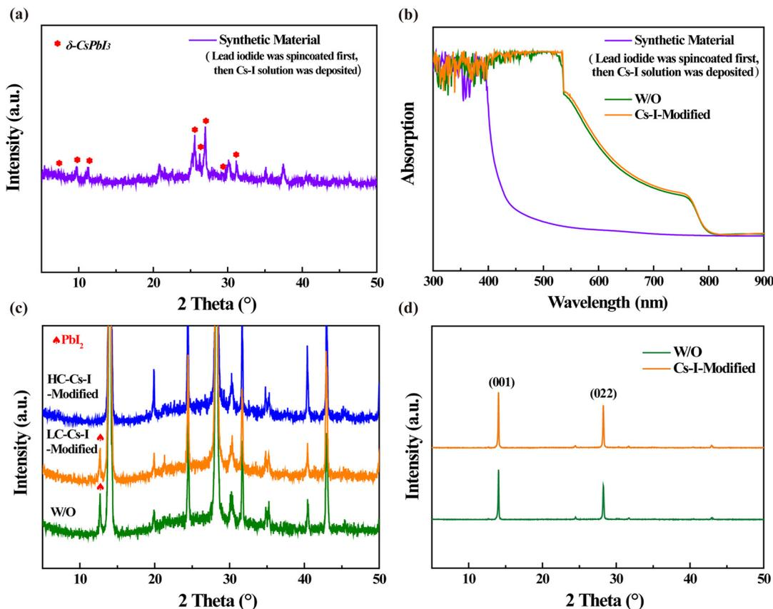
**Fig. 2** (a) XRD patterns of the samples by reacting PbI<sub>2</sub> with equal molar Cs-I precursor solution; (b) UV-visible absorption spectra of the synthetic material, W/O and Cs-I-modified samples. XRD patterns for (c) the reference and films treated with low and high concentrations of the Cs-I precursor and (d) the W/O and Cs-I-modified perovskite films.
