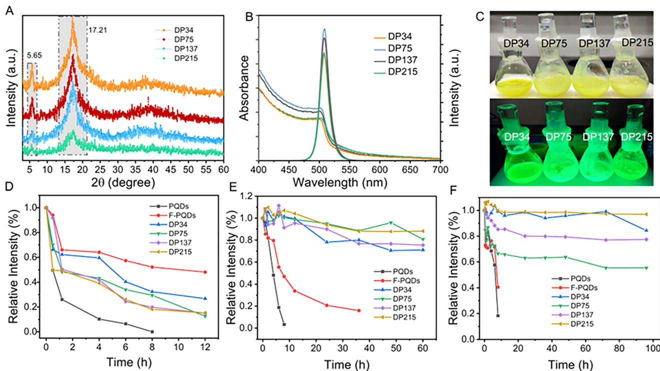
**Fig. 4** (A) XRD spectra, (B) UV-vis absorption spectra and PL spectra, and (C) photographs of different samples. The stability of hybrid nano-assemblies: (D) thermal stability, (E) UV irradiation stability, and (F) polar solvent stability of different samples.
