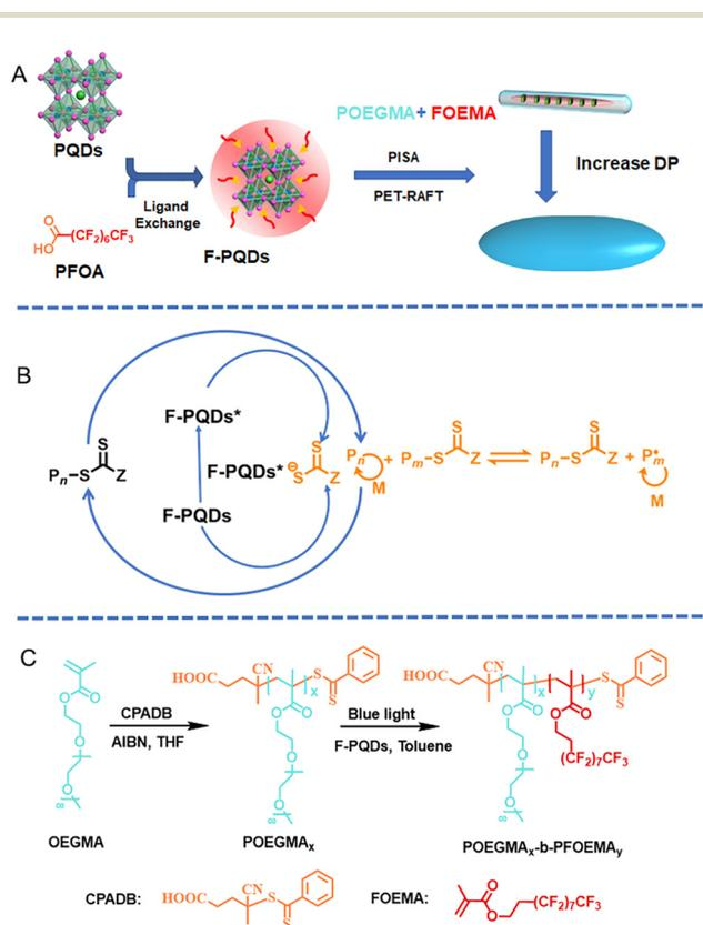
**Scheme 1** (A) Schematic demonstration of the surface ligand exchange strategy of PQDs and the PISA process based on PET-RAFT polymerization, (B) the proposed PET-RAFT polymerization mechanism of F-PQDs, and (C) a synthetic approach for producing the diblock copolymer POEGMA-*b*-PFOEMA.
