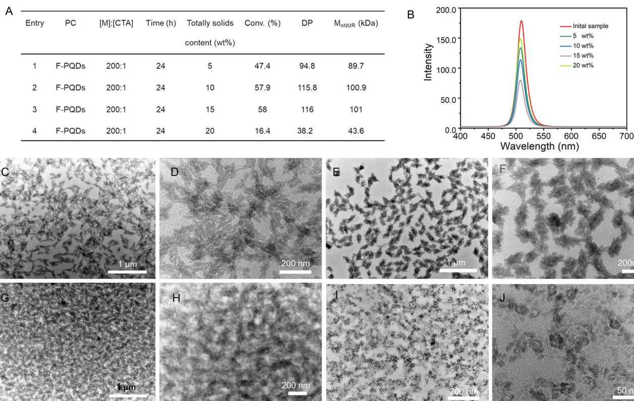
**Fig. 2** (A) Characterization of POEGMA<sub>78</sub>-*b*-PFOEMA diblock copolymers synthesized with a different total solid content, (B) PL spectra (excited at 380 nm) of self-assembled POEGMA<sub>78</sub>-*b*-PFOEMA nanoparticles in toluene, and (C–J) TEM images of self-assembled POEGMA<sub>78</sub>-*b*-PFOEMA nanoparticles.
