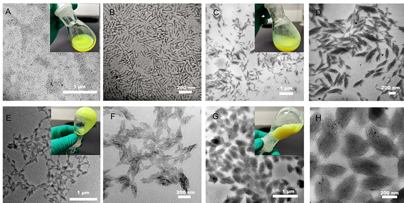
**Fig. 3** TEM images of (A and B) POEGMA<sub>78</sub>-*b*-PFOEMA<sub>34</sub> (conv. = 34%), (C and D) POEGMA<sub>78</sub>-*b*-PFOEMA<sub>75</sub> (conv. = 37.5%), (E and F) POEGMA<sub>78</sub>-*b*-PFOEMA<sub>137</sub> (conv. = 45.6%) and (G and H) POEGMA<sub>78</sub>-*b*-PFOEMA<sub>215</sub> (conv. = 53.7%) (inset: photographs of sample solutions).
