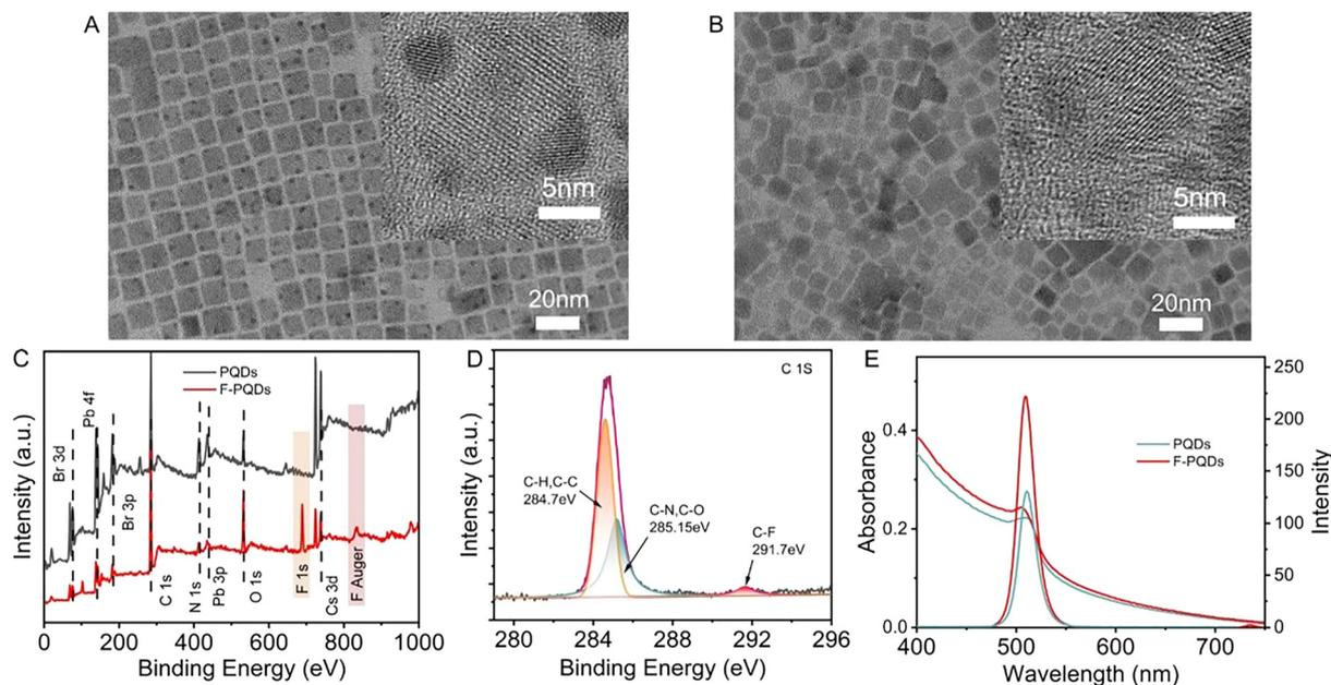
**Fig. 1** (A) TEM and HRTEM images of PQDs, (B) TEM and HRTEM images of F-PQDs, (C) XPS spectra of PQDs and F-PQDs, (D) high-resolution C 1s spectra of F-PQDs, and (E) UV-vis absorption spectra and PL spectra (excited at 380 nm) of PQDs and F-PQDs in toluene.
