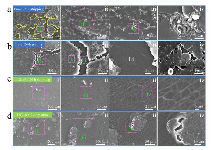
Fig. 7 SEM observations of the morphological changes of Li electrodes: 137 (a and b) bare Li electrode and (c and d) LiGL60 electrode after one 24 h stripping (or plating) at 2 mA cm<sup>-2</sup>. LiGL60 indicates the LiGL coating of 60 MLD cycles. The electrolyte is 1 M LiTFSI in 1/1 volume ratio of DOL/ DME. Reprinted (adapted) with permission from ref. 137 under a Creative Commons Attribution (CC BY) license.
