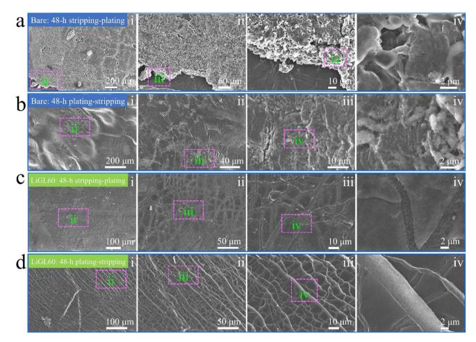
Fig. 8 SEM observations of the morphological changes of Li electrodes: 137 (a and b) bare Li electrode and (c and d) LiGL60 electrode after one 48 h stripping-plating at 2 mA cm<sup>-2</sup>. LiGL60 indicates the LiGL coating of 60 MLD cycles. The electrolyte is 1 M LiTFSI in 1/1 volume ratio of DOL/DME. Reprinted (adapted) with permission from ref. 137 under a Creative Commons Attribution (CC BY) license.
