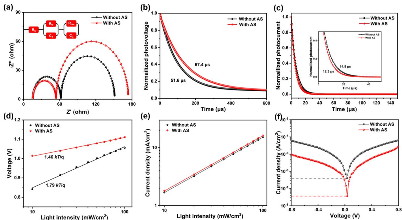
**Fig. 3** (a) Nyquist plot of PSCs fabricated without and with AS methods measured in the dark at  $V \approx V_{oc}$ ; (b) TPV and (c) TPC decay curves of PSCs fabricated without and with AS methods; (d) IMVS and (e) IMPS of PSCs fabricated without and with AS methods; (f) dark current curves of PSCs fabricated without and with AS methods.
