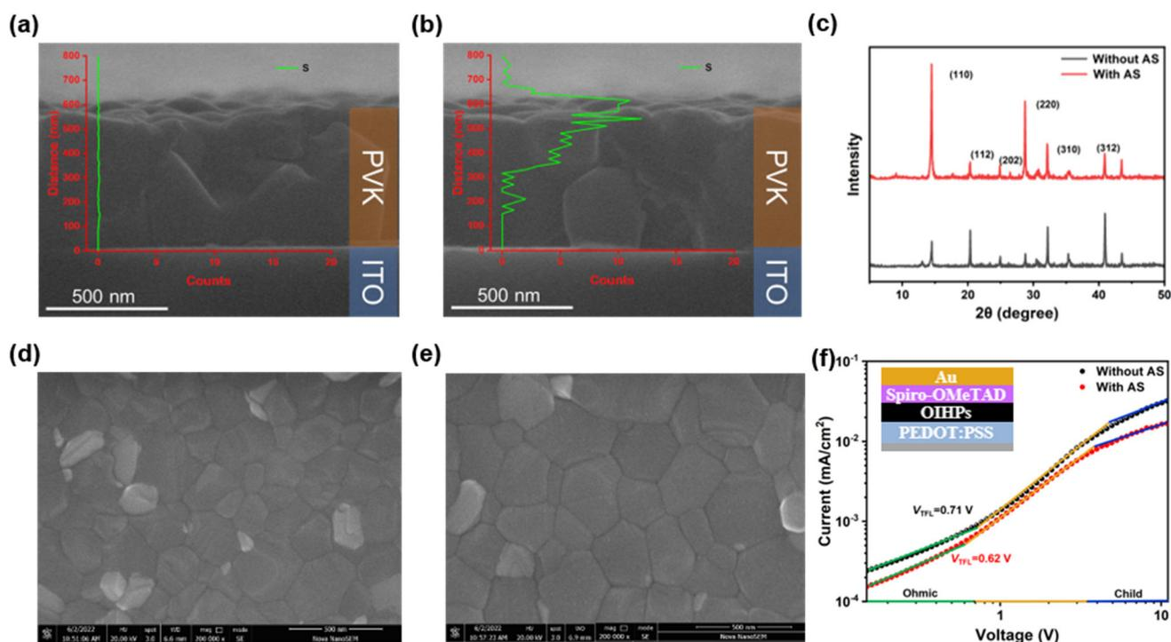
**Fig. 1** Cross-section images and EDS mapping of OIHPs films without (a) and with (b) AS method; (c) XRD patterns of OIHPs films without and with AS method; (d) and (e) were the top SEM of the OIHPs prepared without and with AS method; (f) SCLC curves of pure hole transport devices based on OIHPs prepared without and with AS method.
