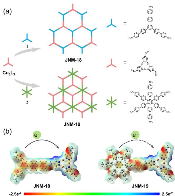
**Fig. 1** (a) Syntheses of imine-linked D–A MOFs, **JNM-18** and **JNM-19**, via Schiff base reactions between the  $\text{Cu}_3$  CTU acceptor ( $\text{Cu}_3\text{L}_3$ ) and TPB (**1**) or HPB (**2**) donors, respectively. (b) The ESP surface maps for the optimized structures of **JNM-18** (left) and **JNM-19** (right). The planar TPB moiety in **JNM-18** shows a stronger electron donating ability than the HPB unit with nonplanar propeller arrangement in **JNM-19**.
