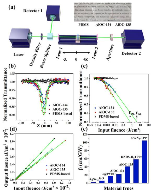
**Fig. 4** (a) Schematic representation of the Z-scan setup (inset is a picture of the PDMS substrate and AIOCs@PDMS under natural light); (b) the OA Z-scan curves of input laser pulse energy 80  $\mu$ J of AIOCs@PDMS; (c) the plots of normalized transmittance versus input fluence; (d) curves of output fluence versus input fluence; and (e) the plots of comparisons of the nonlinear absorption coefficients.
