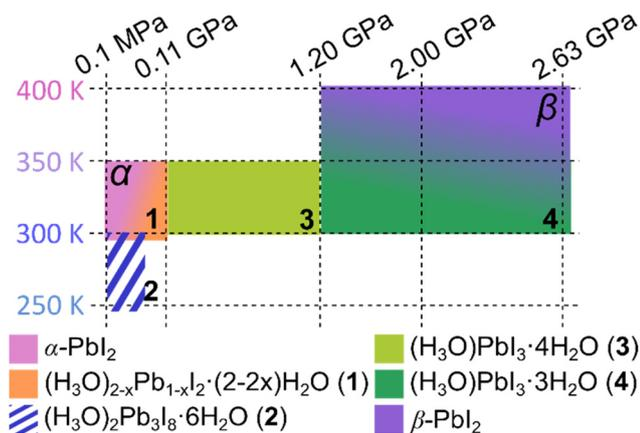
**Fig. 5** The  $p/T$  preference diagram for the  $\text{PbI}_2$  and  $\text{HI}(\text{aq})$  system, with the end members being the previously known 2-D  $\alpha\text{-PbI}_2$  and the herein reported 3-D  $\beta\text{-PbI}_2$ . Acids **1** and **2** are obtained by milling and vapor-solid reactions, whereas **1**, **3**, **4** and  $\beta\text{-PbI}_2$  result from high-pressure synthesis in the DAC.
