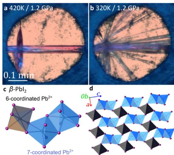
**Fig. 4** The 3-D network polymorph of  $\text{PbI}_2$ . Pink single crystals of  $\beta\text{-PbI}_2$  at 1.2 GPa and: (a) 420 K and (b) 320 K covered by a bundle of needle crystals of **3**. Views of the  $\beta\text{-PbI}_2$  structure: (c) 6- and 7-coordinated  $\text{Pb}^{2+}$  cations shown in grey and blue, respectively, and (d) the 3-D network viewed along the crystallographic  $b$ -axis.
