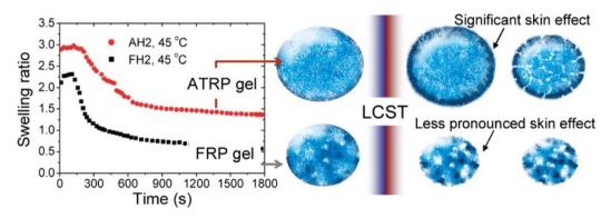
Fig. 3 (Left) Swelling ratio over time for 2-(2-methoxyethoxy)ethyl methacrylate networks above the LCST for both ATRP and FRP networks. Right shows skin like effects on the periphery of the network (reproduced from ref. 75 with permission from American Chemical Society, copyright 2010).
