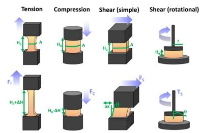
Scheme 9 Typicalmodes of mechanical deformation and testing including tension, compression simple shear and rotational shear. Green arrow shows the direction of the force (F) or torque (T) applied to deform the material, blue highlights the pertinent dimensional parameter. A refers to cross sectional area, r refers to radius,  $H_0$  refers to initial height. Displacements are given as either  $\Delta H$  in tension or compression,  $\Delta x$  in simple shear or  $\theta$  in rotational shear.
