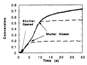
Fig. 1 Double bond conversion *versus* polymerization time for diethyleneglycol dimethacrylate photopolymerized with 110 mW cm<sup>-2</sup> of UV light and 1.0 wt% Irgacure 651. Full cure (solid line) and shutter closed after 3.9 and 9.4 s (dashed line) (reproduced from ref. 61 with permission from American Chemical Society, copyright 1995).
