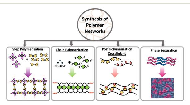
Scheme 1 Different strategies to synthesis of polymer networks using step polymerization in the presence of multifunctional monomers, chain polymerization in the presence of multifunctional monomers, post polymerization crosslinking and phase separation.
