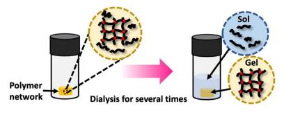
Scheme 7 Gel extraction process: the crosslinked network is dissolved in an appropriate solvent for a specified duration. Subsequently, the weights of the dried sol fraction and gel fraction are measured. Sol-gel fraction is quantified using eqn (1).
