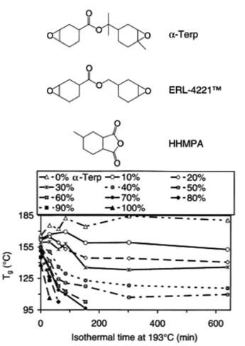
Fig. 7 Glass transition temperatures of the samples used in swelling tests as a function of their rework times. The greater the amount of  $\alpha$ -Terp in the material, the lower the  $T_{\rm g}$  (reproduced from ref. 105 with permission from Elsevier, copyright 2004).
