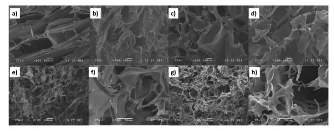
Fig. 9 SEM images of HEC<sup>90</sup>/AAc hydrogels (M<sub>v</sub> = 90 000) containing (a) 5% (b) 10% (c) 20% and (d) 30% AAc. HEC<sup>1300</sup> (e and f) and HEC<sup>1300</sup>/AAc gels ( $M_v = 130\,000$ ) containing 5% AAc (g and h) (magnification: x100ae and g; x500f and h) (reproduced from 115 with permission from Elsevier, copyright 2017).
