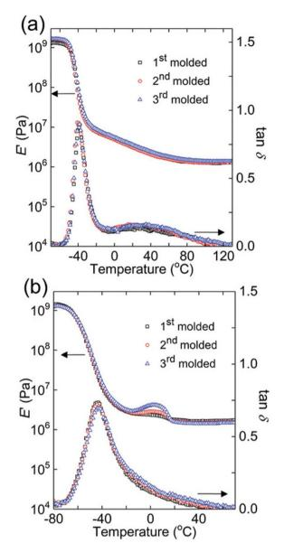
**Fig. 8** Dynamic mechanical responses of (a) PB networks and (b) PTMO networks: E' and  $\tan \delta$  as functions of temperature for 1st molded (squares), 2nd molded (circles), and 3rd molded (triangles) samples (reproduced from ref. 112 with permission from John Wiley and Sons, copyright 2019).
