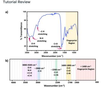
Scheme 6 (a) Schematic diagram of a typical IR spectrum, (b) schematic representation of regions where the major bonds normally absorb.
