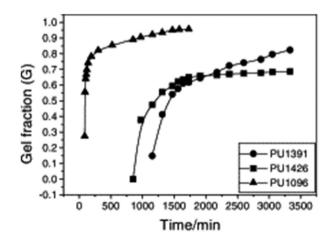
Fig. 2 Dependence of gel fraction on the curing time of PU at room temperature (reproduced from ref. 50 with permission from Elsevier, copyright 2000).
