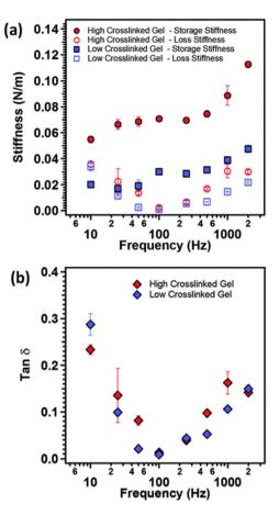
Fig. 10 (a) The storage modulus (closed symbols), loss modulus (open symbols) and (b)  $\tan \delta$  as function of modulation frequency of the AFM cantilever for polyacrylamide gels with two different crosslinking densities (reproduced from ref. 127 with permission from Royal Society of Chemistry, copyright 2015).
