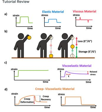
Scheme 11 (a) Schematic of stress response to strain applied to a perfectly elastic (blue) and perfectly viscous (red) material, (b) conceptual demonstration of viscoelasticity in the context of a ball dropped (image inspired by slide 15 from ref. 89), (c) schematic response of a viscoelastic material to applied strain in a stress relaxation experiment. (d) Schematic response of a viscoelastic material to a transiently applied stress in a creep experiment.
