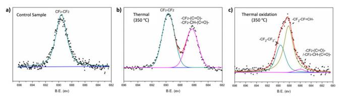
Fig. 11 High-resolution XPS spectra of the F 1s of FEPM vulcanizate (a) before, (b) after thermal aging and (c) under thermal oxidation conditions (adapted with modifications from ref. 139 with permission from Elsevier, copyright 2020).
