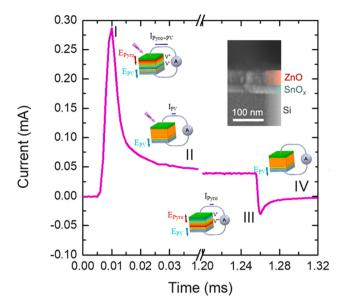
**Fig. 17** Time response of an ITO/ZnO/SnO<sub>x</sub>/Si/Al-based self-powered device with insets indicating four stages and a schematic. Copyright "Elsevier", 2021 (included with permission).
