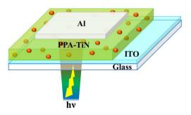
**Fig. 26** Schematic of PPA-TiN-based hybrid photodetector. <sup>152</sup> Copyright "American Chemical Society", 2016 (included with permission).
