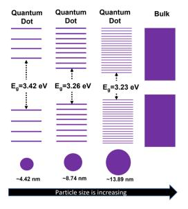
**Fig. 8** Demonstration of variation of the bandgap of quantum dots (QDs) with respect to the size of the QDs. <sup>59</sup>
