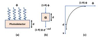
Fig. 3 (a) Schematic of a photodetector showing incident flux  $(\phi)$ , (b) illustration of incident intensity with respect to an absorption coefficient ( $\alpha$ ), and (c) illustration of variation due to absorbed energy in a photodetector.
