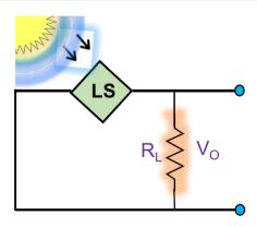
Fig. 1 Self-powered photodetector.
