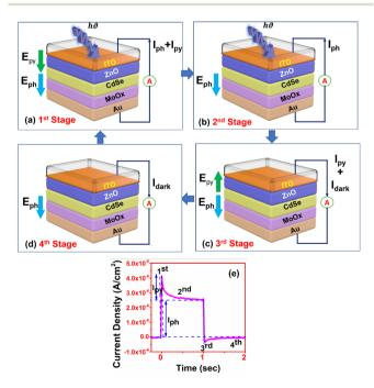
**Fig. 16** (a–d) Four stages of pyro-phototronic effect, and (e) time response, of an ITO/ZnO QD/CdSe QD/MoO<sub>x</sub>/Au-based self-powered photodetector.<sup>115</sup>
