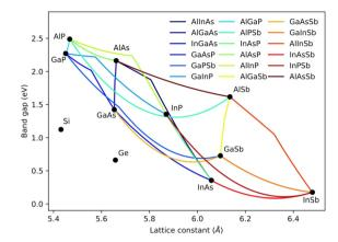
Fig. 9 Variation of bandgap with lattice constant in different alloyed materials, 67 Published by "Springer Nature" as open access, 2018.
