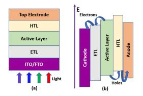
Fig. 6 (a) Schematic of a photodetector with back illumination utilizing an ETL and an HTL, (b) energy band diagram of the photodetector.
