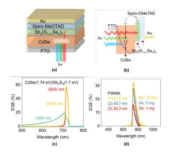
Fig. 13 (a) Schematic of the self-powered photodetector, (b) schematic of carrier transport in the device, (c) EQE for different CdSe thicknesses, and (d) EQE for different Se concentrations.<sup>83</sup> Published by "Wiley-VCH" as open access, 2021.
