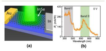
Fig. 25 (a) Schematic, and (b) responsivity versus wavelength of the plasmon-based InSe/Au dual-band self-powered photodetector. 151 Copyright "American Chemical Society", 2018 permission).
