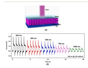
**Fig. 18** (a) Schematic of an ITO/ZnO NW/PEDOT:PSS/Ag-based device. (b) Time response for different nanowire lengths. Copyright "Elsevier", 2022 (included with permission).
