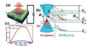
**Fig. 14** (a) Schematic of a graphene/Si nanohole array Schottky junction based self-powered near-infrared photodetector, (b) energy band diagram of the device with and without surface passivation under light, and (c) responsivity with and without surface passivation for different wavelengths. Published with "Optica Publishing Group" as open access, 2015.
