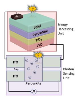
Fig. 5 Schematic of a photodetector-solar cell-based nanosystem. 16
