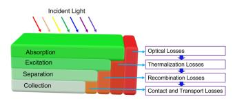
Fig. 2 Photodetection process and associated losses.
