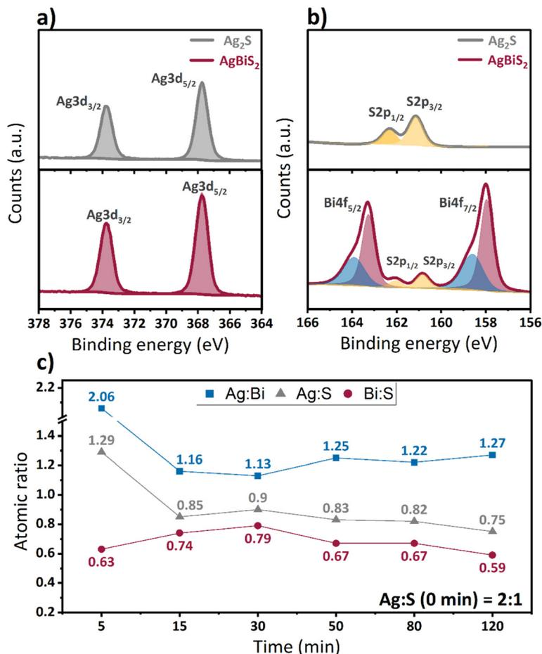
Fig. 4 XPS spectra of (a) Bi 4f and S 2p, (b) Ag 3d for Ag<sub>2</sub>S and AgBiS<sub>2</sub> QDs after cation exchange of 120 min. (c) Comparison of the atomic ratio between Ag, Bi, and S at different cation exchange times.
