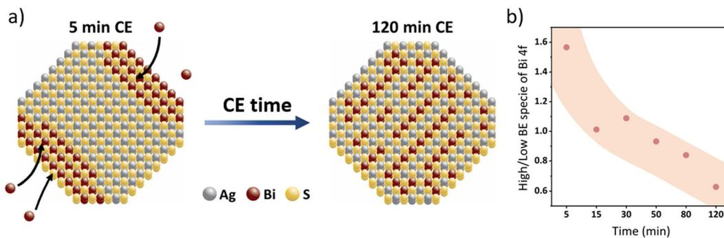
**Fig. 6** (a) Schematic representation of the cation exchange process and resulting homogenization of the cation disorder with increasing reaction time, (b) evolution of the ratio between high-binding/low-binding energy Bi species with CE time.
