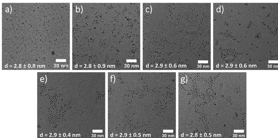
Fig. 2 TEM images of (a)  $\text{Ag}_2\text{S}$  QDs before and during the cation exchange at (b) 5 min, (c) 15 min, (d) 30 min, (e) 50 min, (f) 80 min, and (g) 120 min of reaction time. Scale bar 30 nm (bottom right) and average QD size and standard deviation (bottom left) for each image.
