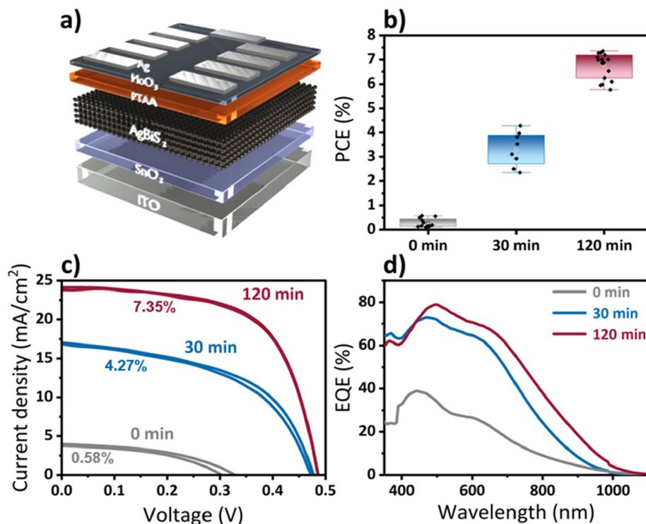
**Fig. 5** (a) Schematic device architecture of AgBiS<sub>2</sub> solar cells, (b) Solar cell performance (PCE) of AgBiS<sub>2</sub> QDs obtained after different times of cation exchange, (c) *J*–*V* curves (forward and reverse scanning) of devices with different QDs after 0 min (Ag<sub>2</sub>S), and AgBiS<sub>2</sub> after 30 min, and 120 minutes of cation exchange with individual PCE (d) corresponding EQE curves for these three devices.
