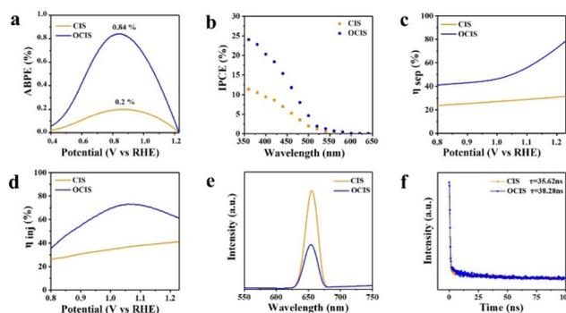
**Fig. 4** (a) ABPE and (b) IPCE for CIS and OCIS. (c) Charge separation efficiency and (d) charge injection efficiency of CIS and OCIS. (e) Steady-state PL spectra for CIS and OCIS with excitation wavelength  $\lambda_{ex}$  = 325 nm. (f) TRPL decay spectra for CIS and OCIS.
