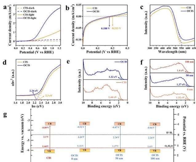
**Fig. 3** (a) LSV curves and (b) onset potentials for CIS and OCIS. (c) UV-vis absorption spectra and (d) corresponding Tauc plots for CIS and OCIS. (e) VB-XPS spectra for CIS and OCIS. (f) VB-XPS spectra for OCIS with different etching depths. (g) Energy level diagram for CIS and OCIS with gradient oxygen doping.
