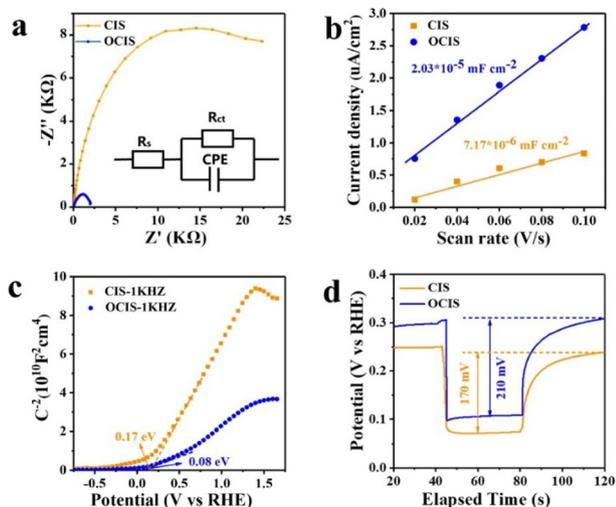
**Fig. 5** (a) The EIS Nyquist plots for CIS and OCIS under illumination. (b) Current densities of CdIs of CIS and OCIS. (c) M–S plots for CIS and OCIS in dark. (d) OCP measurements under dark and light conditions for CIS and OCIS.
