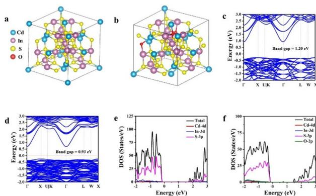
**Fig. 6** Side view of (a) bulk  $\text{CdIn}_2\text{S}_4$  and (b) bulk  $\text{CdIn}_2\text{S}_4$  with three S atoms replaced by O atoms. Band structure of (c) CIS and (d) OCIS. Density of states of (e) CIS and (f) OCIS.
