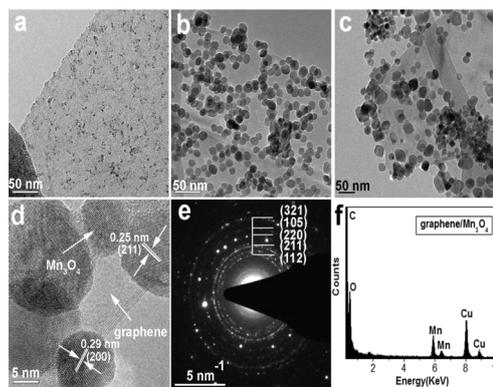
Fig. 12 TEM analysis of graphene/ $\text{Mn}_3\text{O}_4$  NCs: products prepared at reaction times of 4 h (a), 8 h (b), and 16 h (c); HRTEM image of attached  $\text{Mn}_3\text{O}_4$  NPs (d) and corresponding SAED pattern (e); and (f) EDS pattern of  $\text{Mn}_3\text{O}_4$  NPs. Reproduced with the permission from ref. 246. Copyright 2017, the Royal Society of Chemistry.
