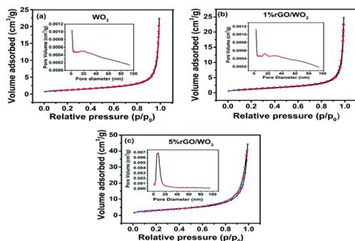
Fig. 13 Nitrogen-adsorption/desorption isotherms and corresponding pore size distribution of (a) pure  $\text{WO}_3$ , (b) 1% rGO/ $\text{WO}_3$  and (c) 5% rGO/ $\text{WO}_3$ . This figure has been reproduced from ref. 247 with permission from the Royal Society of Chemistry, Copyright 2019.
