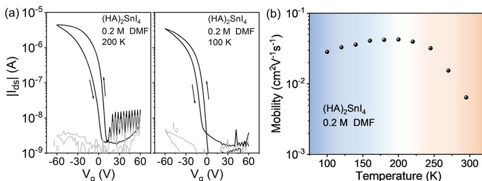
Fig. 6 Low temperature transfer characteristics of the  $(\text{HA})_2\text{SnI}_4$ -based FET device at (a) 200 and 100 K. (b) Corresponding temperature-dependent field-effect mobility from 100 K to 295 K.
