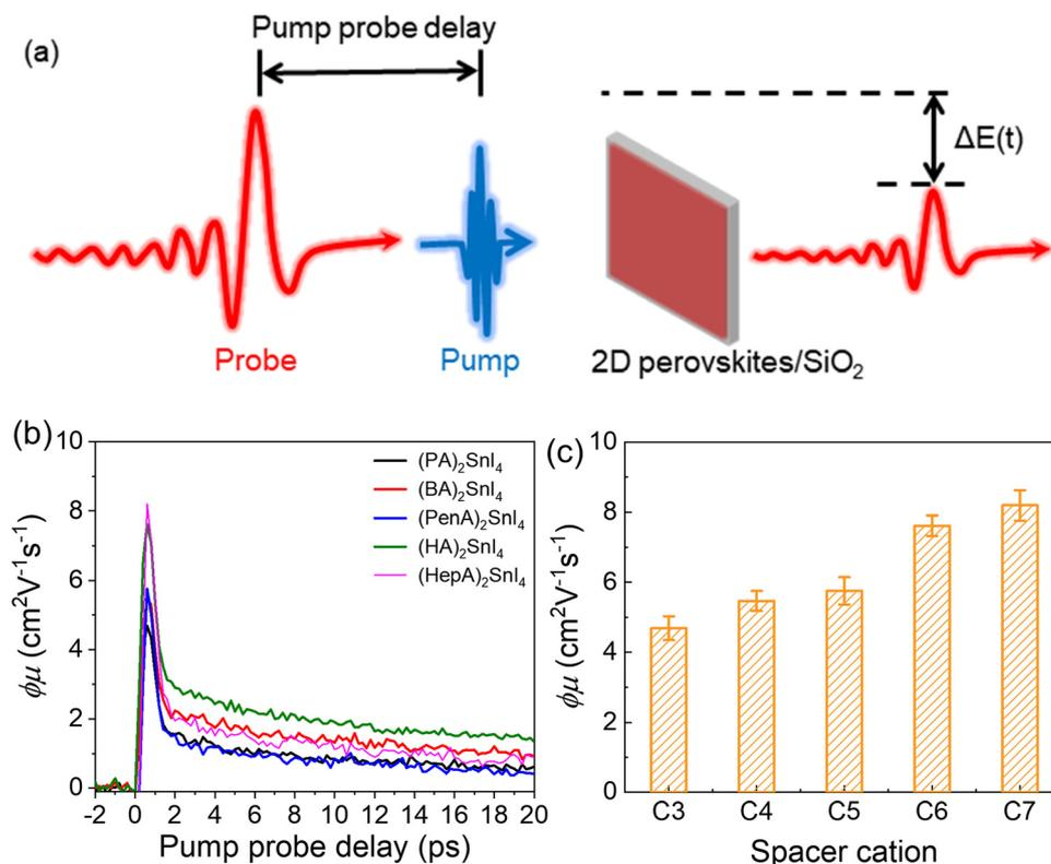
Fig. 4 (a) Photoconductivity dynamics by optical pump–THz probe (OTPT) spectroscopy. (b) Comparison of the mobility and free-carrier generation quantum efficiency ( $\phi_\mu$ ) for the five perovskites. (c) Charge carrier mobility (peak values in a) as a function of the chain length of the spacer cation.
