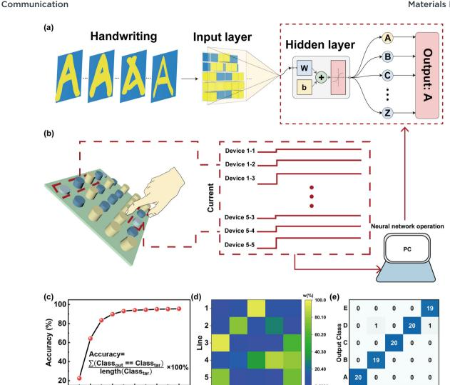
Fig. 6 (a) A schematic of handwriting recognition based on in-sensor computing. (b) The structure and working principle of the humidity in-sensor handwriting recognition system. (c) The accuracy of handwriting recognition. (d) The weight of  $5 \times 5$  array after handwriting. (e) The confusion graph of the output class and the target class about handwriting letters of alphabet "A," "B," "C," "D," and "E" after 40 cycles.
