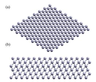
(a) Top view and (b) side view of Al(1 1 1) surface. A total of 6 layers of Al were used in this calculation. The grey circles represent aluminum
