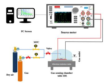
Illustration of the gas detection system.
