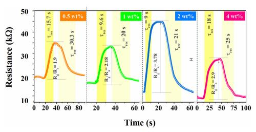
Fig. 8 Effect on NO<sub>2</sub> sensing behavior with variation in rGO concentration (0.5-4 wt%)
