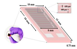
Thin film-based sensor fabrication over IDE
