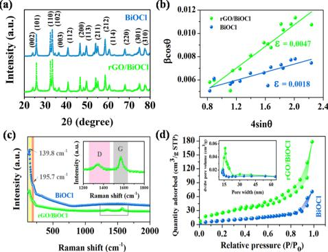
Fig. 4 (a) XRD peaks pattern, (b) Williamson-Hall plot, (c) Raman spectra and (d) N<sub>2</sub> sorption isotherm for pristine BiOCl and rGO/BiOCl along with the pore size distribution curve (inset).
