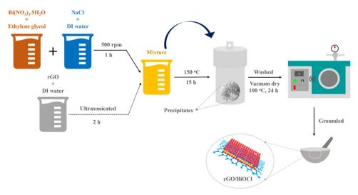
Fig. 1 Synthesis route for rGO/BiOCl heterostructure.
