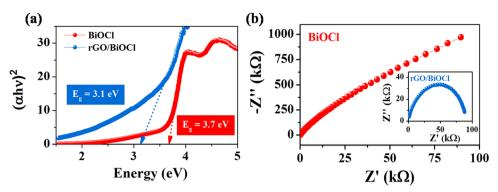
Fig. 6 (a) Tauc plot and (b) EIS spectra for pristine BiOCl and rGO/BiOCl.
