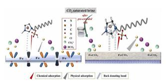
Fig. 20 Protective mechanism of DMIMHS towards the corrosion inhibition of Fe and FeCO<sub>3</sub> surface. [Reprinted with permission from ref. 119, @2022 Elsevier.]
