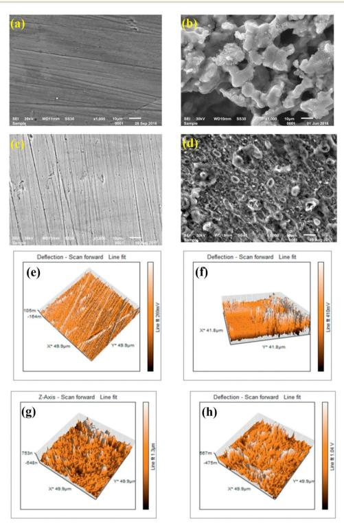
Fig. 13 SEM (a–d) and AFM (e–h) images of (a and e) the polished mild steel, (b and f) after immersion within 0.5 M  $\rm H_2SO_4$  without IL, (c and g) with  $10^{-2}$  M [FBMIm]Br, and (d and h) with  $10^{-5}$  M [FBMIm]Br. [Reprinted with permission from ref. 126, ©2019 Elsevier.]
