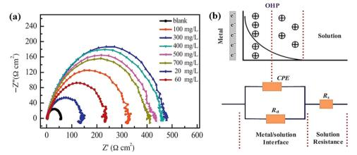
Fig. 6 (a) Nyquist plot for the carbon steel working electrode in the presence of  $0.1 \,\mathrm{M}\,\mathrm{H}_2\mathrm{SO}_4$  solution without and with different concentrations of BKC, (b) potential distribution diagram at the interface between the metal and the electrolytic solution (above) and analogous circuit used to fit the Nyquist plot (bellow) [reprinted with permission from ref. 95, ©2015 Elsevier].
