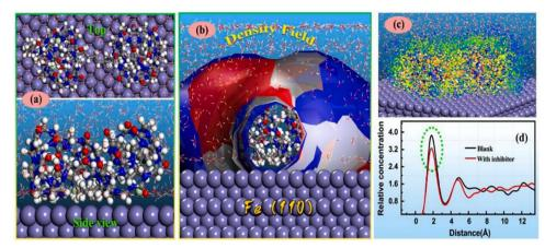
Fig. 21 (a) Optimized adsorption configuration of CB6-based [3] rotaxane on the Fe(110) surface, (b) density field distribution, (c) concentration distribution analysis, and (d) concentration distribution of water. [Reprinted with permission from ref. 97, ©2022 Elsevier.]
