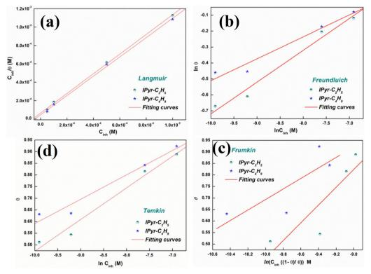
Fig. 10 (a) Langmuir, (b) Freundluich, (c) Frumkin and (d) Temkin isotherm models for understanding the adsorption mechanism of IPyr-C<sub>2</sub>H<sub>5</sub> and IPyr-C<sub>4</sub>H<sub>9</sub> on mild steel surface in the presence of 1 M HCl at 298 K. [Reprinted with permission from ref. 103, ©2020 Elsevier.]
