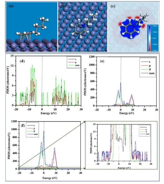
Fig. 15 (a) Side view, (b) top view, (c) charge density difference plot of the equilibrium adsorption configuration of 1-butylpyridinium cation on Fe(110) surface; partial density of states (PDOS) of (d) 1-butylpyridinium cation, (e) iron surface and (c) 1-butylpyridinium cation after adsorption on Fe(110) surface. [Reprinted with permission from ref. 35, @2023 Elsevier.]
