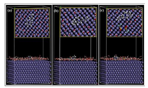
Fig. 16 Side view of the optimized adsorption configuration of (a) IL-1; (b) IL-2 and (c) IL-3 on the Fe(110) plane in a simulated acid medium (i.e., in the presence of 150 H<sub>2</sub>O, 15H<sub>3</sub>O<sup>+</sup> and 15Cl<sup>-</sup>) obtained from MD simulation (inset: top view). [Reprinted with permission from ref. 100, ©2021 Elsevier.]
