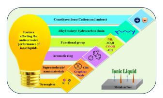
Fig. 5 Key factors that regulate the corrosion inhibition performance
