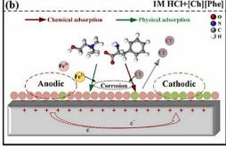
Fig. 17 Schematic representation of the (a) corrosion mechanism of mild steel in the presence of 1 M HCl and (b) corrosion inhibition mechanism of mild steel in the presence of [Ch][Phe] in 1 M HCl solution. [Reprinted with permission from ref. 99, ©2023 Elsevier.]
