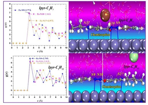
Fig. 18 RDF analysis of adsorbed lpyr-C3H7 and lpyr-C5H11 on Fe(110) surface in a simulated acid medium at 298 K temperature obtained from MD simulation. [Reprinted with permission from ref. 104, ©2021 Elsevier.]
