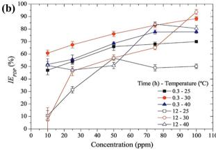
Fig. 7 After evaluating API-X52 steel as a working electrode in the presence of 1 M HCl solution, the inhibition efficiency of (a) TMA and (b) TTA as functions of the immersion duration and temperature [reprinted with permission from ref. 90, @2018 Elsevier].
