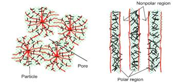
Fig. 6 Illustration of the polarity distribution between disordered (left) and more oriented nanofibers (right).15
