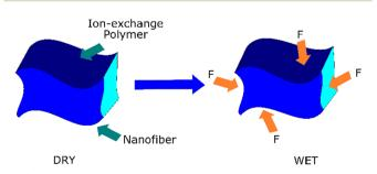
Fig. 8 Mechanism of the nanofiber suppressing the swelling of the matrix.<sup>92,93</sup>
