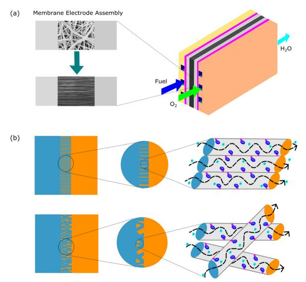
Fig. 5 (a) The idea of transforming a random nanofiber into an aligned nanofiber implemented in the membrane electrode assembly in fuel cells. (b) Comparison of aligned structures and isotropic fibres based on their transport function.
