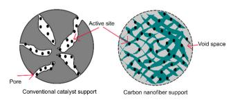
Fig. 7 Comparison of a conventional porous support (left) and carbon nanofiber support (right).
