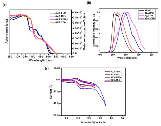
Fig. 2 (a) Normalized absorption and molar extinction coefficient spectra and (b) photoluminescence spectra of aza-[7]helicenes in dry CHCl<sub>3</sub> solution. (c) Cyclic voltammetry spectra of aza-[7]helicenes in dry DCM solution.
