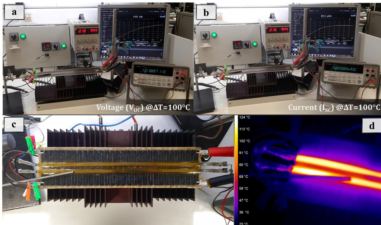
Fig. 7 GFRP-GTEG-device performance at  $\Delta T$ : 100 °C: (a) the generated open-circuit voltage ( $V_{OC}$ ) and, (b) the short-circuit current ( $I_{SC}$ ). (c) Thermoelectric power measurement set-up and (d) thermal image of the testing performance.
