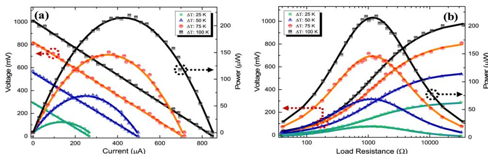
Fig. 6 The thermoelectric performance of the GFRP-GTEG as evaluated experimentally in various  $\Delta T$ s. (a) The obtained curves of voltage–current ( $V-I$ ), power–current ( $P-I$ ) and (b) voltage–load resistance ( $V-R_{\text{load}}$ ), power–load resistance ( $P-R_{\text{load}}$ ).
