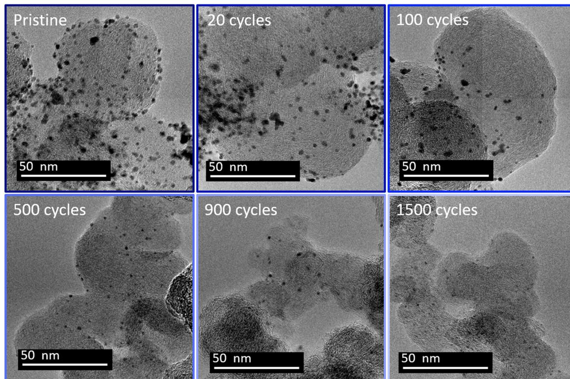
Fig. 3 Representative TEM images of platinum particles from a Pt/C 20% TTK at 20  $\mu\text{g cm}^{-2}$  loading at different stages of cycling between 1.2 and 0.85 V *vs.* RHE in 1 M H<sub>2</sub>SO<sub>4</sub> + 0.01 M NaCl.
