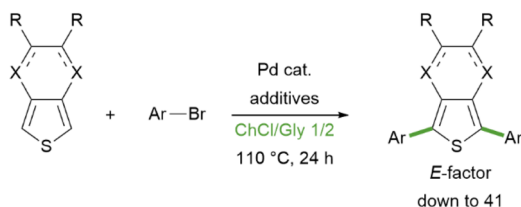
Scheme 1 Previous report on the direct C–H arylation of EDOT (X = O, R = H, single bonds) or TP (X = N, R ≠ H, double bonds) with aryl bromides in the ChCl/Gly DES. 25
