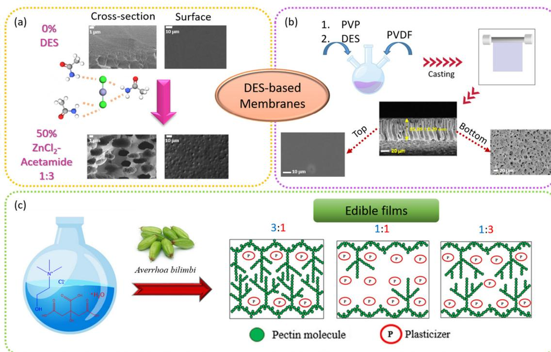
**Fig. 10** Illustration of the generation of porous membranes and their SEM images. (a) Polyamide-imide membranes before and after incorporation of  $\text{ZnCl}_2$ :acetamide.<sup>164</sup> Copyright 2021, MDPI. (b) With non-ionic DES (*N*-methyl acetamide:*N*-methyl urea).<sup>165</sup> Copyright 2022, Elsevier. (c) Schematic illustration of the plasticization effect of edible films generated by *Averrhoa bilimbi* pectins with a DES.<sup>175</sup> Copyright 2020, Elsevier.
