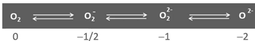
Fig. 1 Oxygen redox chemistry showing transition via addition of electrons from dioxygen gas (O 2 ) to superoxide (O 2 − ) to peroxide (O 2 2− ) to oxide (O 2− ), with the formal oxidation number written below.
