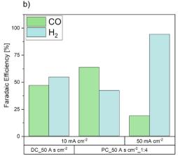
Fig. 5 Electrochemical performance of the electrodeposited electrodes compared to the sputtered electrode. (a) Linear sweep voltammetry measurements for GDEs deposited with a charge density of 50 A s cm $^{-2}$ , (b) faradaic efficiency of the detected CO<sub>2</sub>RR products after 1 h of operation (b).
