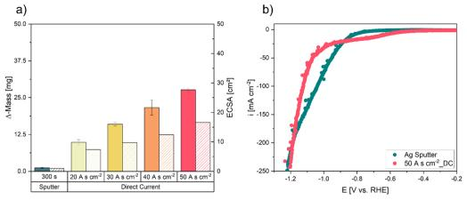
Fig. 3 Characterization of the Aq-sputtered electrode compared to the DHBT electrodes manufactured in DC mode. (a) Deposited Aq mass and ECSA values of Ag-sputtered electrode and DHBT foam electrodes with increasing charge densities during DC mode, (b) linear sweep voltammetry curves for the Ag sputter electrode and the DC-50 A s cm<sup>-2</sup> electrode to test their electrochemical performance (IR corrected potentials by applied CI method).
