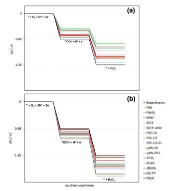
Fig. 10 Free-energy diagrams at 0 V vs. RHE for hydrogen peroxide production on the ideal catalyst using several xc-functionals. (a) Gasphase corrections are not included. (b) Only the errors in  $O_2$  are corrected. In black in both panels is the experimentally expected profile, obtained when both errors are corrected. Reproduced from ref. 27, licensed under CC BY 4.0 (https://creativecommons.org/licenses/by/4.0/).
