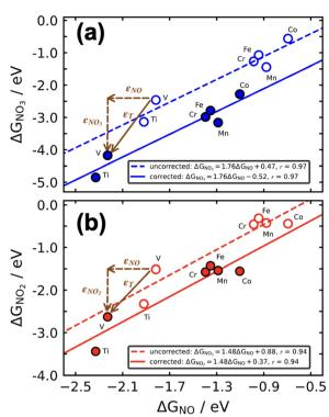
Fig. 15 Free energies of adsorption of \*NO<sub>3</sub> (a) and \*NO<sub>2</sub> (b) versus that of \*NO on metalloporphyrins. Dashed lines and open circles correspond to uncorrected energies, solid lines and solid circles correspond to energies upon gas-phase corrections. Brown vectors on the V-containing porphyrin show the displacements introduced by the respective gas-phase errors. Reproduced from ref. 29, licensed under CC BY 4.0 (https:// creativecommons.org/licenses/by/4.0/)
