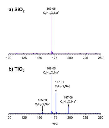
Fig. 6 High-resolution mass spectra of extracted products from (a)  $SiO_2$  and (b)  $TiO_2$  surfaces following a 30 min DMS exposure followed by 1 h evacuation. Ions are shown as sodium adducts.
