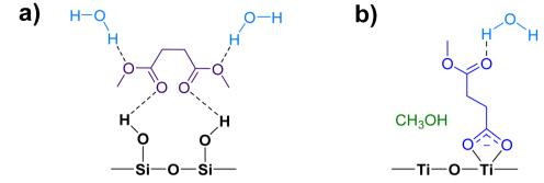
Fig. 9 Interactions of water molecules with adsorbed DMS species on (a) SiO<sub>2</sub> and (b) TiO<sub>2</sub> surfaces
