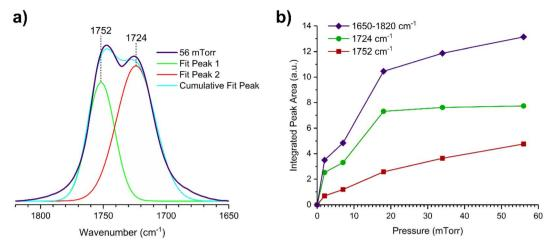
Fig. 2 (a) Deconvoluted carbonyl peaks of the SiO<sub>2</sub> surface after DMS exposure at 56 mTorr. (b) Integrated FTIR peak areas as a function of pressure (mTorr) of the entire carbonyl band (1650 to 1820 cm<sup>-1</sup>) and the deconvoluted peaks (at 1724 and 1752 cm<sup>-1</sup>).
