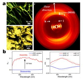
**Fig. 13** (a) POM and SAXS images system **4-9**. (b) CPL and  $g_{lum}$  spectra of **4-9** films under different states. Reproduced from ref. 104 with permission. Copyright (2020), American Chemical Society.
