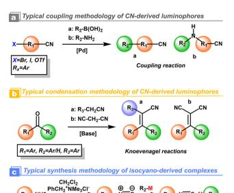
Scheme 2 Schematic representation of synthesis methodologies for polar cyano/isocyano-derived luminophores.  $R_x$  represents aryl groups.
