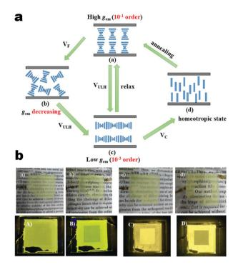
**Fig. 11** (a) Schematic illustration of thermo-electric-induced CPL switching, LC assembly model for system **4-6**. (b) Images of N\*-LCs-**4-6** system device under enhanced DC electric field. Reproduced from ref. 98 with permission. Copyright (2022), The Royal Society of Chemistry and the Chinese Chemical Society.
