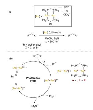
Scheme 6 (a) Che's seminal work using  $[(\mu-dppm)_2Au_2]^{2+}$  (dppm = bis (diphenylphosphino)methane), and (b) common proposed mechanism involving complex 28.
