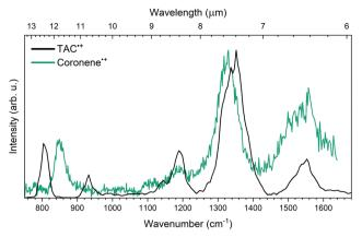
Fig. 5 Experimental IRMPD of TAC<sup>•+</sup> (black) and coronene<sup>•+</sup> (green). Both spectra are normalized with respect to their most intense peak. The IRMPD spectrum of coronene<sup>•+</sup> is taken from Oomens et al.<sup>22</sup>
