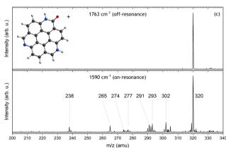
Fig. 2 Mass spectra of isolated TAC<sup>++</sup> (a), TACH<sup>++</sup> (b) and [TAC-H + H<sub>2</sub>O]<sup>++</sup> (c) after exposure to off-resonance (top panel) and on-resonance (bottom panel) infrared radiation. The wavenumber of the IR radiation is depicted in each respective panel. The proposed geometry for the  $[TAC-H + H_2O]^+$ species is discussed in Section 3.4.
