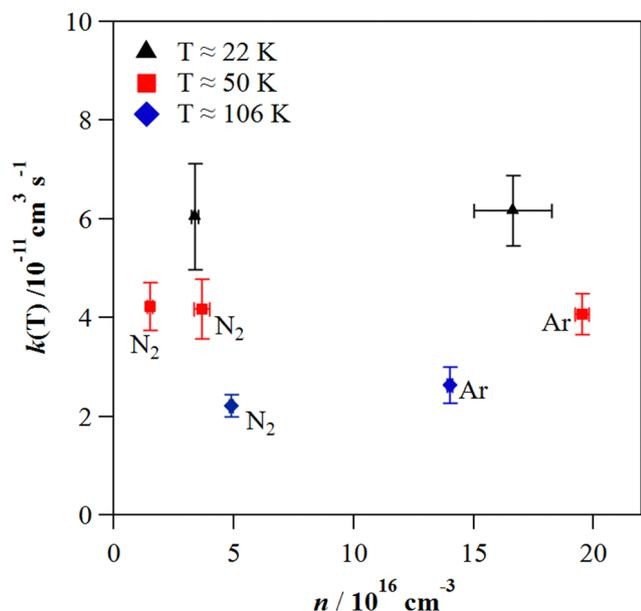
Fig. 3 Dependence of  $k(T)$  on the jet gas density ( $n$ ) at ca. 22, 50, and 106 K. Black triangles correspond to experiments at 22 K in He, while at 50 and 106 K the bath gas is indicated next to each point. Error bars in  $k(T)$  are statistical ( $\pm 2\sigma$ ) and 10% systematic errors and in  $n$  are only statistical ( $\pm\sigma$ ).
