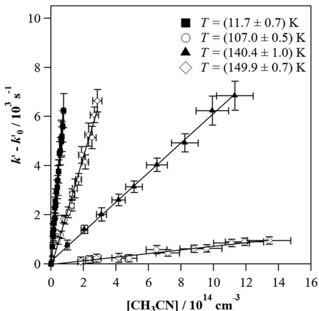
Fig. 1 Examples of  $k' - k'_0$  versus  $[\text{CH}_3\text{CN}]$  plots at four different temperature conditions. Uncertainties in  $[\text{CH}_3\text{CN}]$  are cautiously considered as  $\pm 10\%$  and uncertainties in  $k' - k'_0$  are the standard deviation obtained from the analysis of the  $I_{\text{LIF}}$  decays.
