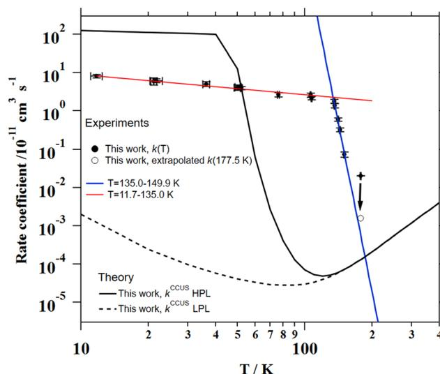
Fig. 4 Experimental and theoretical temperature dependence of the rate coefficient for the  $\text{CH}_3\text{CN} + \text{OH}$  reaction. Red and blue lines represent the resulting fit to  $k(T) = A (T/300 \text{ K})^n$  in the stated temperature range. Solid and dashed black curves are the computed HPL and LPL rate coefficients.
