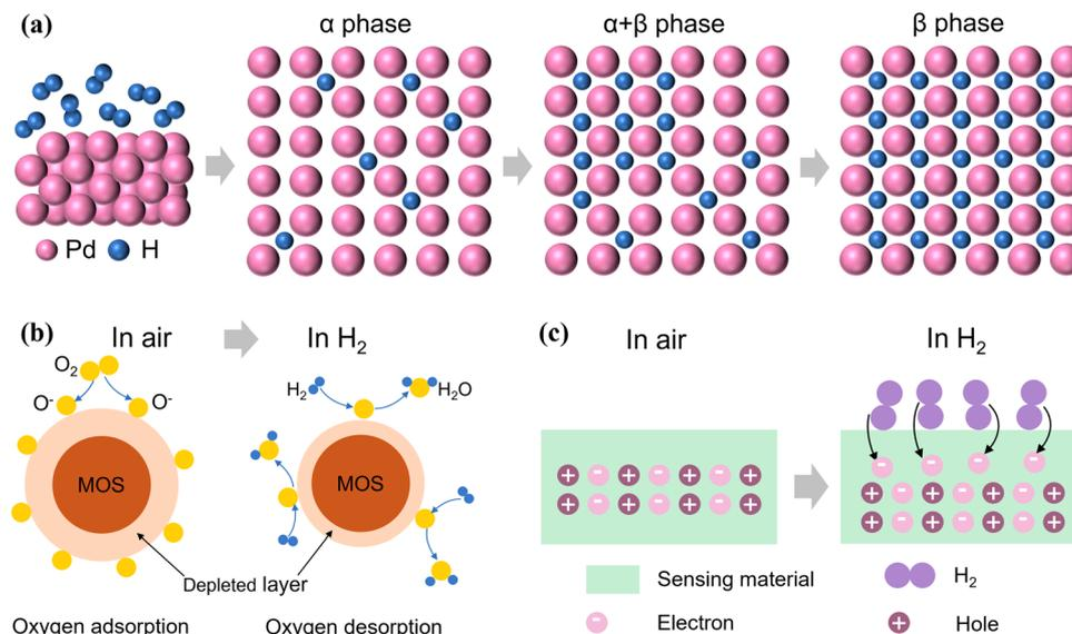
Fig. 1 (a) Schematic of hydrogen diffuse into the Pd lattice. (b) Schematic of chemisorption based on MOSs. (c) Schematic of physisorption.
