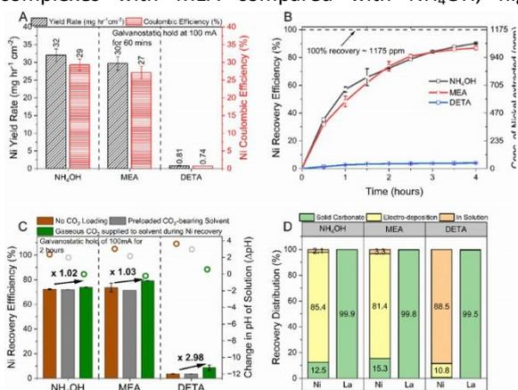
**Fig. 3 (a)**, Ni yield rate and coulombic efficiencies in different  $\text{CO}_2$  capture solvents at galvanostatic hold of 100 mA for 1 hr. **(b)** Comparison of Ni recovery efficiency as a function of time for  $\text{NH}_4\text{OH}$ , MEA and DETA **(c)** The effect of  $\text{CO}_2$  loading on Ni recovery efficiency. **(d)** Integrated experiments showing distribution of products as carbonates, electrodeposition material and unrecovered metal.
