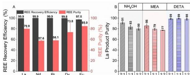
**Fig. 2.** (a) Recovery efficiencies and product purity for REE/Ni separation using NH<sub>4</sub>OH at REE:Ni of 1:2. (b) The product purity at different concentration ratios for NH<sub>4</sub>OH, MEA and DETA.
