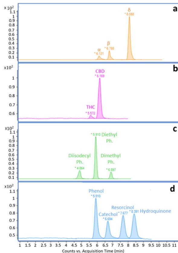
**Fig. 3** (a–d). NPLC MRM and SIM reconstructed ion chromatograms of the selected model compounds: (a) tocopherols; (b) cannabinoids; (c) phthalates; (d) phenols. Analytical conditions are reported in Table 1.
