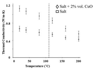
Fig. 18 Experimental data showing elevation in thermal conductivity before and after addition of CuO nanoparticles to NaNO<sub>3</sub>–KNO<sub>3</sub>. Adapted from ref. 34, with permission from Elsevier, Copyright 2016.
