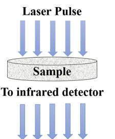
**Fig. 13** Schematic diagram of the laser flash method. Adapted from Open Access data under the Creative Commons BY license from ref. 69, Copyright 2021 MDPI.
