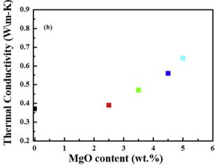
Fig. 20 Experimental data showing the thermal conductivity of NaNO $_3$ -KNO $_3$  (a) improves with the addition of MgO at different mass concentrations (2.5%, 3.5%, 4.5% and 5%) with temperature, and (b) the increasing thermal conductivity at different concentrations. Adapted from ref. 35, with permission from Elsevier, Copyright 2020.
