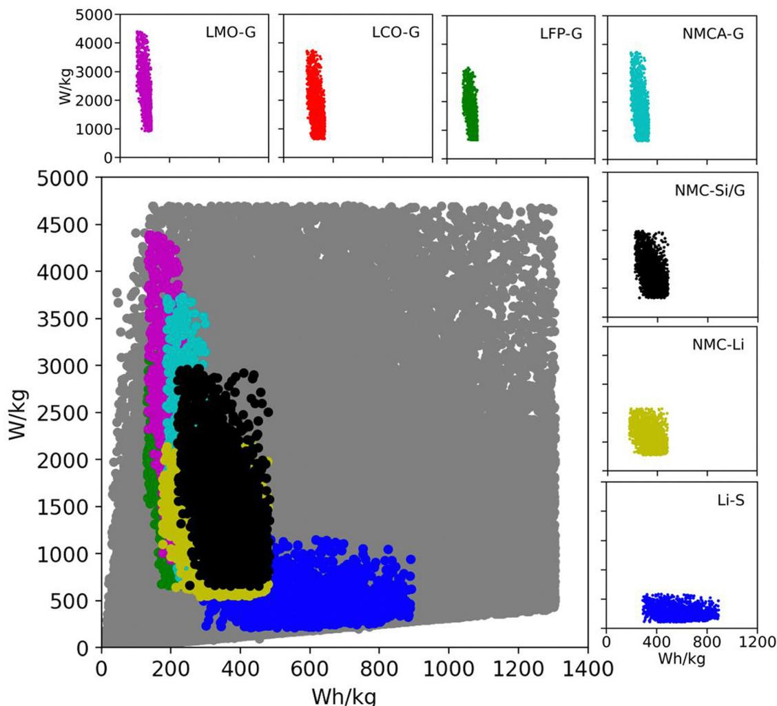
Fig. 2 Ragone space as spanned by the database generated from 200 000 Monte Carlo simulations in BatPaC.<sup>12</sup> The gray points correspond to the entire dataset spanned by the variable ranges in Table 2. The colored subspaces correspond to data spanned by commercial and emerging lithium-ion technologies whose variable ranges are listed in Table S4 (ESI†).
