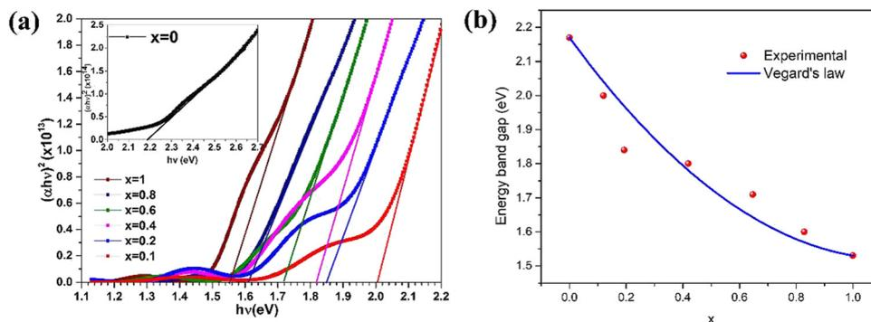
**Fig. 7** (a) Tauc plots where vertical scale bears unit  $(\text{cm}^{-1} \text{eV})^2$  and (b) variation in optical energy band gap as a function of Zn content for Cd<sub>1-x</sub>Zn<sub>x</sub>Te thin films. Reprinted from ref. 119 with permission, Copyright (2020), Elsevier Ltd.
