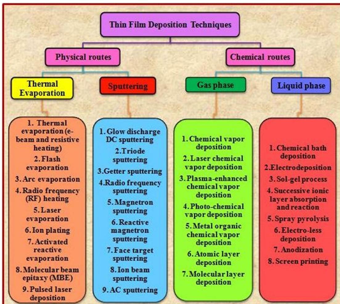
Fig. 3 Overview of the various thin film deposition techniques.<sup>49</sup>
