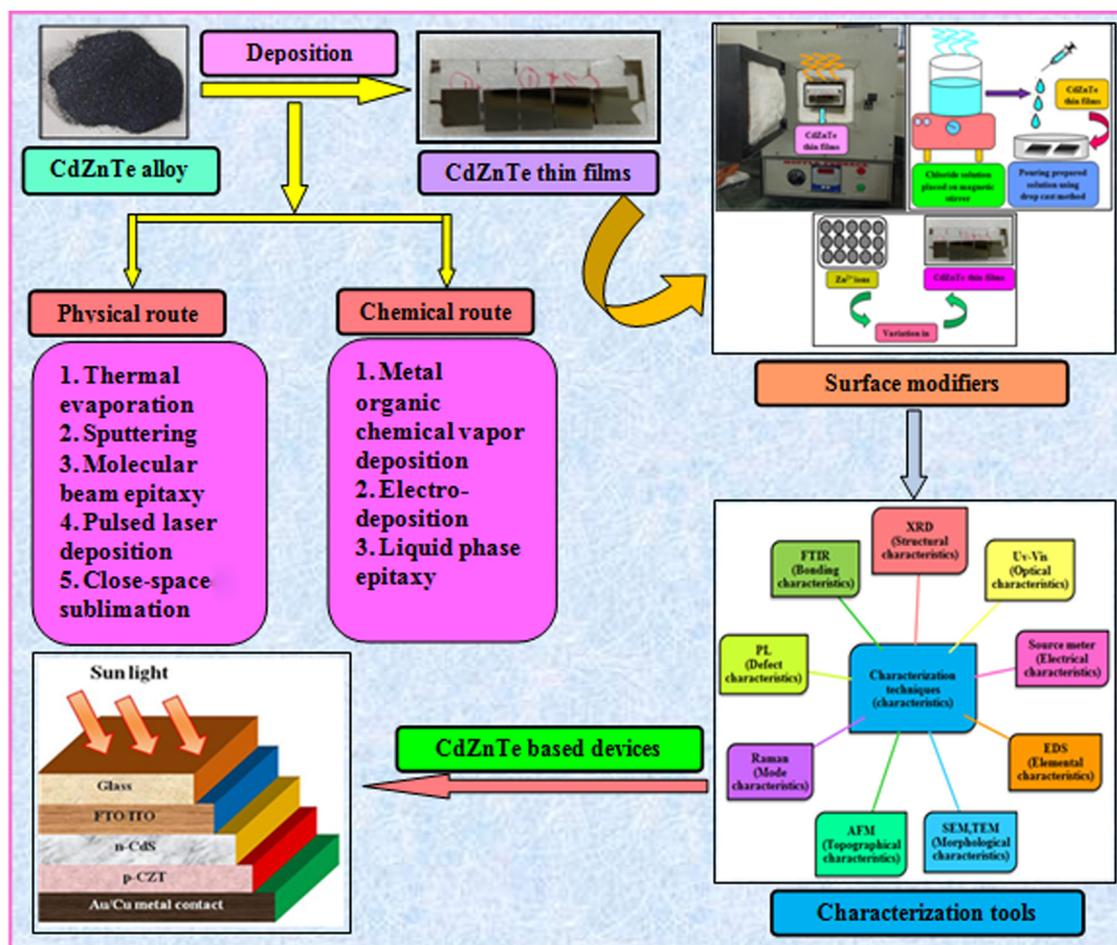
**Fig. 1** Pictorial illustration of the various experimental tools used for the deposition and characterization of CdZnTe thin films, surface modifiers and the CdZnTe-based solar cell device architecture.
