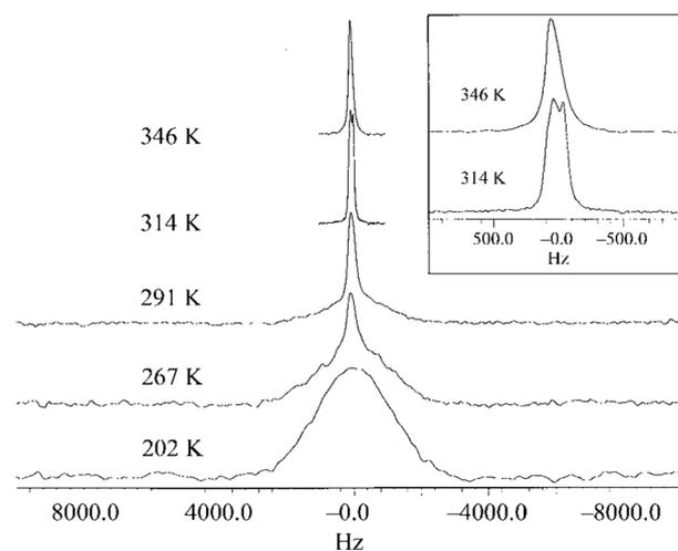
Fig. 5 <sup>7</sup>Li NMR spectra for 9.3 mol% LiTFSA in **1a**, as a function of temperature. The inset is an expansion of the peaks for 314 K and 346 K. Reprinted from ref. 29 with permission.
