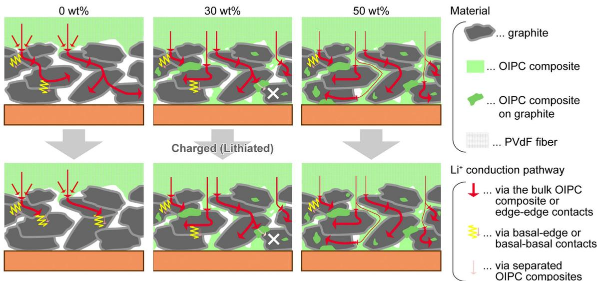
Fig. 11 Role of OIPC in the solid-state electrodes. Mixing OIPC with graphite anode promotes  $\text{Li}^+$  conduction and electrochemical reaction in the electrode layer. Reprinted from ref. 115 with permission.
