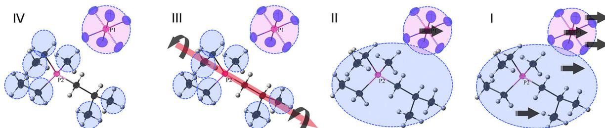
Fig. 7 Schematic of molecular motions in different phases (IV to I) of **26f** with increasing temperature. Phase IV, only the methyl and ethyl groups of the cation are rotating, but the anion is tumbling (on the NMR time scale); phase III, the whole cation can rotate around one axis, and the anion continues tumbling; phase II, the whole cation can tumble, and the anion both tumbles and diffuses; phase I, both the cation and the anion can diffuse. Reprinted from ref. 33 with permission.
