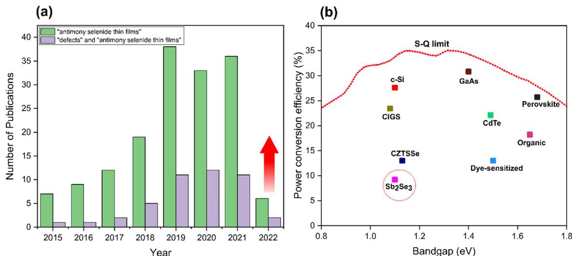
Fig. 1 (a) The number of publications regarding  $\text{Sb}_2\text{Se}_3$  thin-film solar cells and defects analysis of  $\text{Sb}_2\text{Se}_3$  thin-film solar cells from 2015 to 2022 (data extracted from Web of Science). (b) Peak reported single junction efficiencies for different absorber materials in comparison to the S–Q limit.
