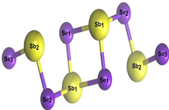
Fig. 3 Non-equivalent atomic sites in  $[\text{Sb}_4\text{Se}_6]_n$  atomic chain.
