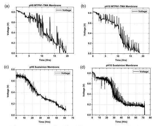
Fig. 9 Durability data for (1) mTPN1-TMA membranes at (a) pH-9 (b) pH-10 (2) Sustainion membranes at (c) pH-9 (d) pH-10 at a constant current density of 0.15 A  $cm^{-2}$
