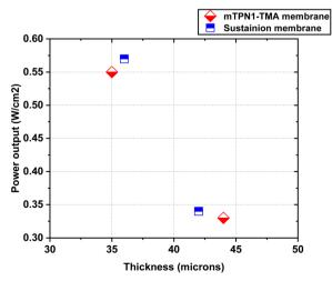
Fig. 12 Power output of both mTP1-TMA membranes and sustainion membranes at different thickness caused by pH.
