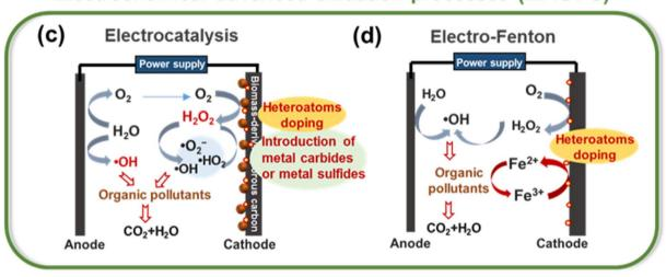
Fig. 2 Working mechanisms of (a) photocatalysis, (b) sulfate radical-based advanced oxidation processes, (c) electrocatalysis and (d) electro-Fenton via bio-based IHPC catalysts. Information regarding the aforementioned mechanisms was adopted from ref. 13, 73, 76, 86 and 90.
