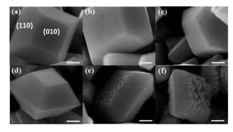
Fig. 2 SEM images of  $BiVO_4$  samples etched in NaOH solution with different concentrations. (a) 0 M; (b) 0.1 M; (c) 0.2 M; (d) 1.0 M; (e) 2.0 M and (f) 3.0 M. Scale bar, 500 nm.
