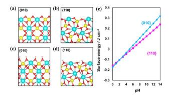
Fig. 1 Theoretical simulation of the (a) {010} facet, (b) {110} facet, (c) hydrogen-rich (010) facet and (d) hydrogen-rich (110) facet of decahedron BiVO<sub>4</sub>. (e) Effect of the pH value on the stability of the hydrogen-rich (010) and (110) facets of decahedron BiVO<sub>4</sub>.
